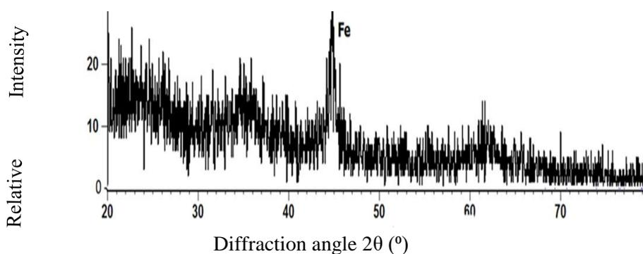
**Fig. 2:** The X-ray pattern of NZVI reveal an apparent peak at the diffraction angle  $2\theta$  value of  $45^\circ$ , which indicated the formation of Nano-iron in the Zerovalent state ( $\text{Fe}^0$ ).
