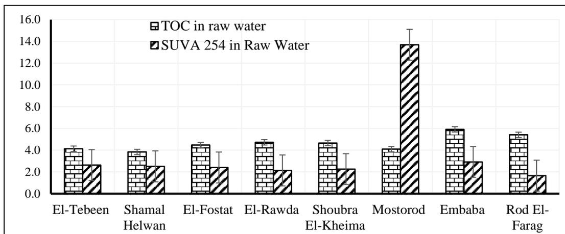
Figure 1: TOC (mg/l) and SUVA<sub>254</sub> (L/mg. m) in raw water
