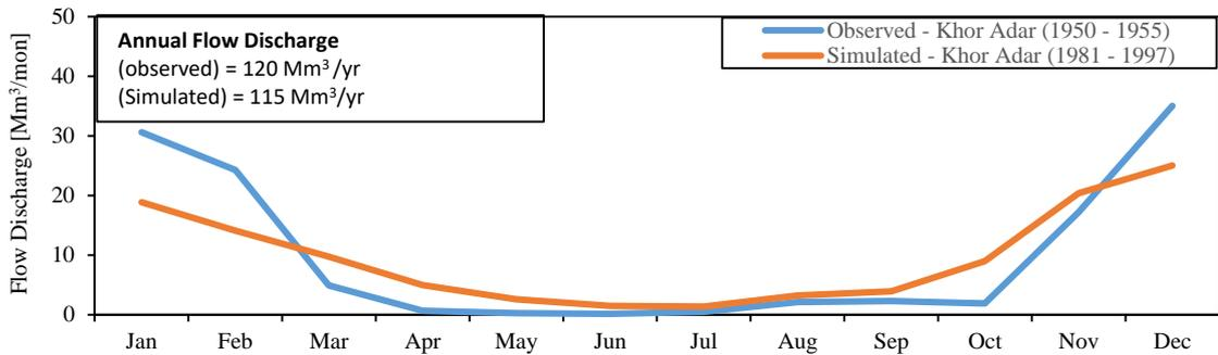
**Figure 1. Comparison of the observed and simulated mean monthly discharge at Khor Adar – Machar Marshes.**
