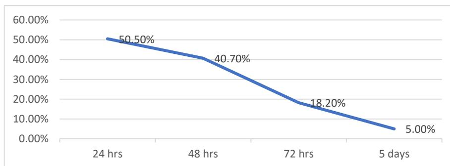
**Figure 2. Green removal of lead by *Aspergillus niger*.**
