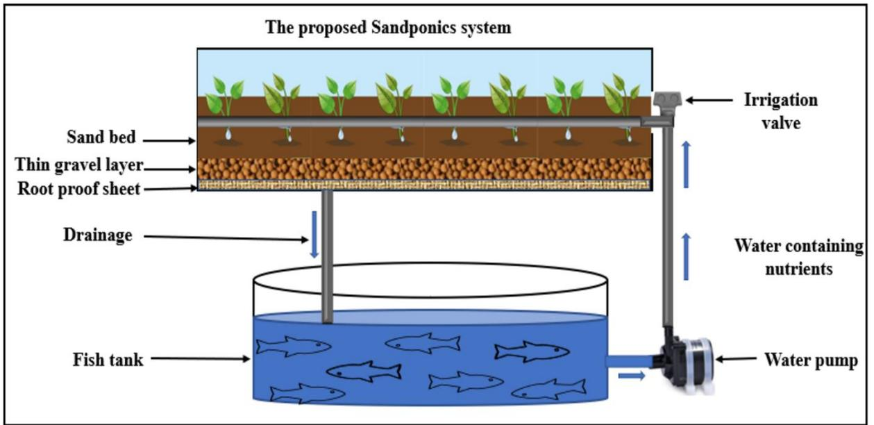
Figure 1. Schematic design of the experimental layout.
