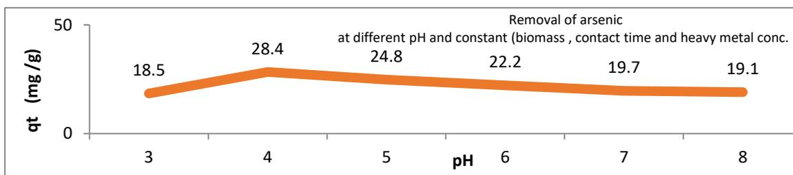
**Fig. 1. Effect of pH on biosorption of arsenic by the dried microalgae *Chlamydomonas* sp. at constant time 60 min, biosorbent dose 1 gm/l, temperature 25 °C and heavy metal concentration 50 mg/l.**
