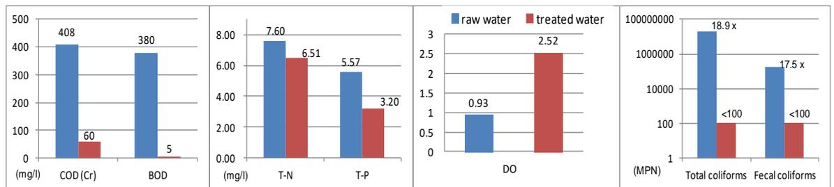
**Figure 1: Comparison of water quality before/after the treatment (Rural sewerage treatment facility) in Sandala Village in Kafr Elshiekh Gov**
