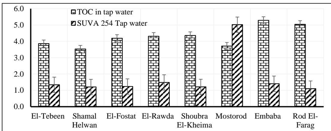
Figure 2: TOC (mg/l) and SUVA<sub>254</sub> (L/mg. m) in tap water
