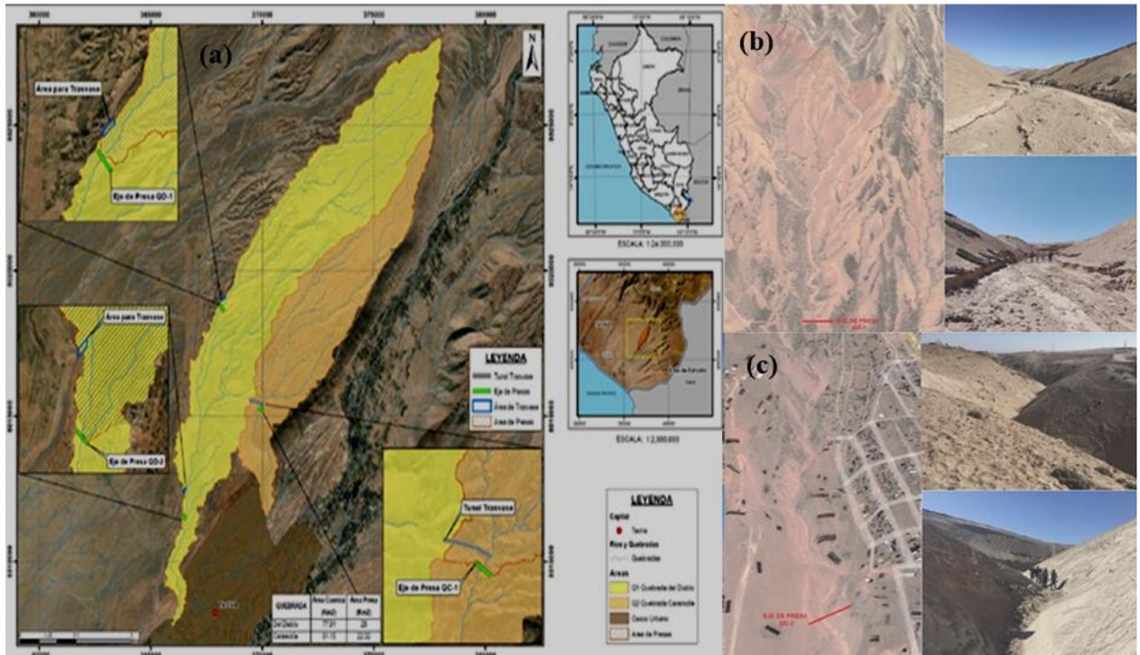
**Figure 2. (a) Approach to alternative structural measures for the comprehensive control of landslides affecting Tacna. (b) View of the axis of the QD-1 (left). (c) QD-2 (right) dam for landslide control and the solids storage vessel.**
