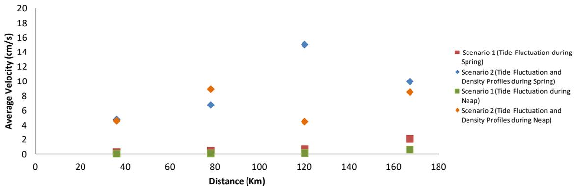
**Figure 1. Extracted model average flow velocity over 200m depth at different locations along the basin of tidal only and tidal/density currents at selected random time. Note station 0.0 is at the basin northern tip location.**
