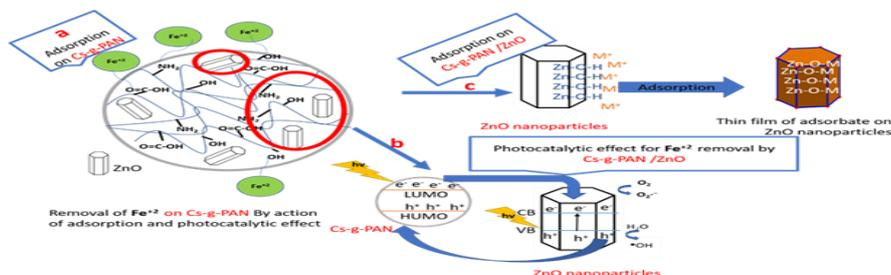
**Scheme 1: Mechanisms for removal of Fe(II) by Cs-g-PAN/ZnO**
