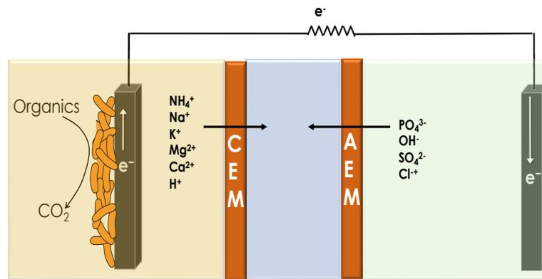
Figure 1. Schematic diagram of microbial nutrient recovery cell used in this study
