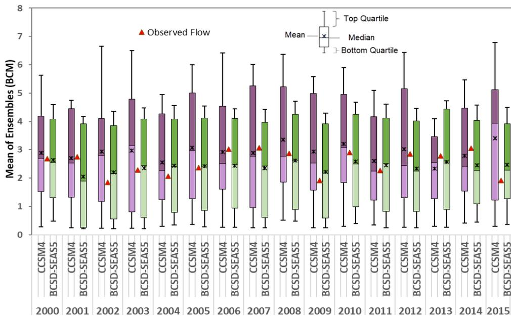
**Figure 1. 10 days boxplot of the mean ensemble of forecasted flow and the mean of observed flow for the LT6 at Diem station**
