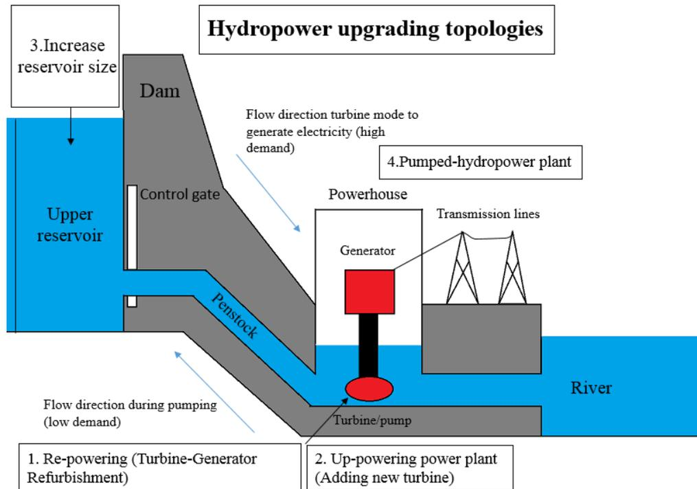
**Figure 1: Hydropower upgrading topologies**
