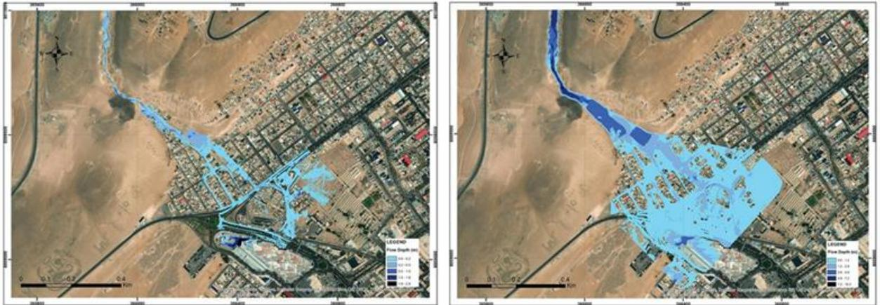
**Figure 1. Flow depth output overlaid with a satellite image of the affected area for the no embankment condition (left). Maximum Flow Depths of the February 21, 2020 Event Reenactment (right)**
