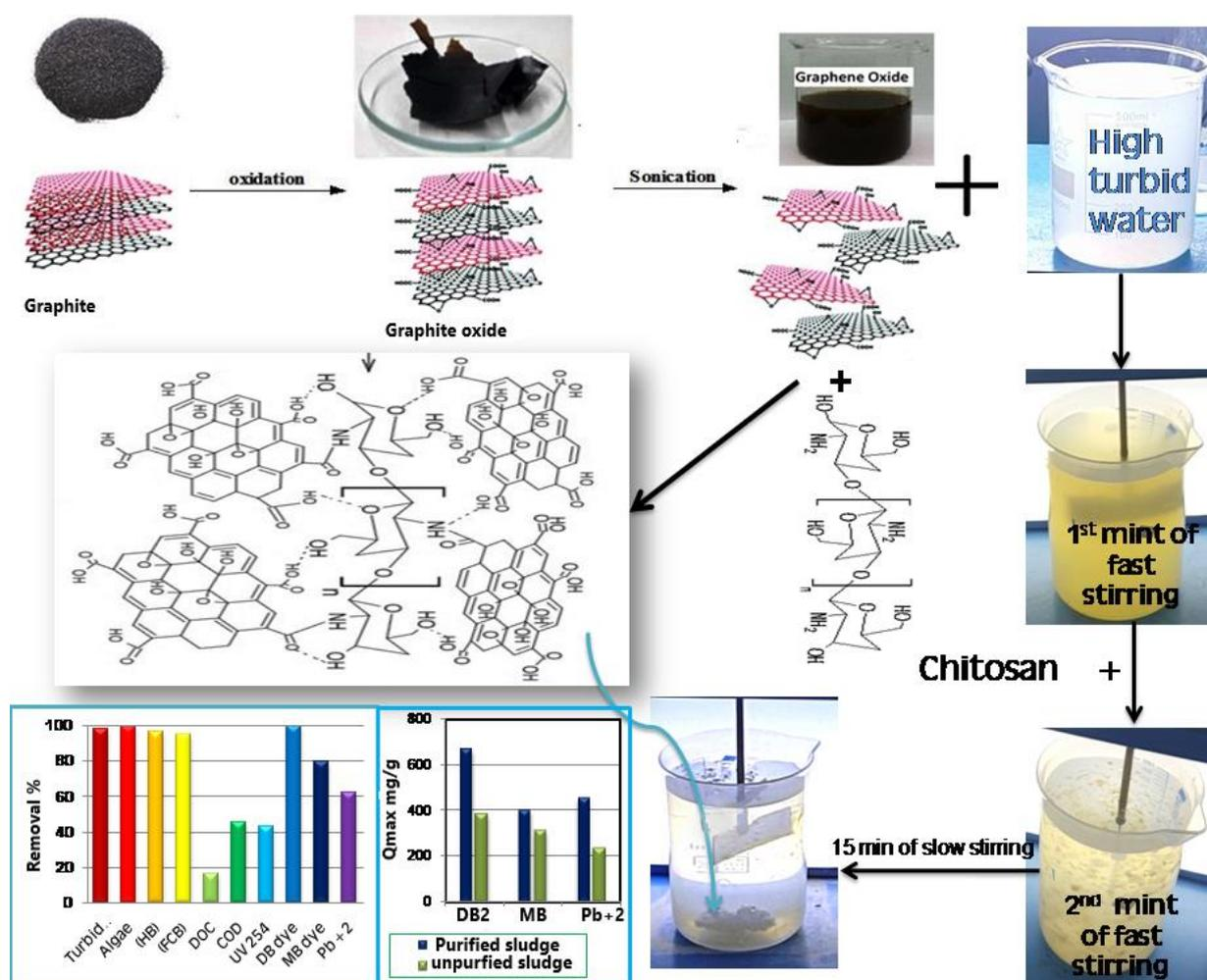
Figure 1: Graphical abstract shows the diverse steps during coagulation/flocculation process by GO/CS up to the last minute of the process beside its impact on various pollutants.
