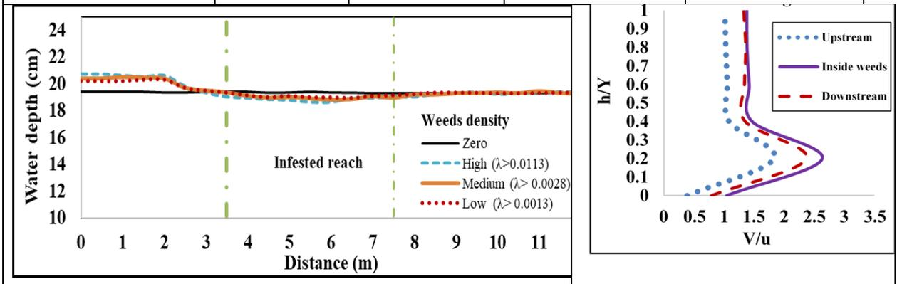
**Figure 1. Sample for water surface profile and vertical velocity profile results**
