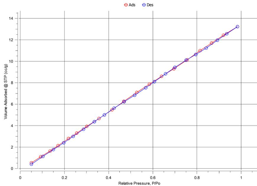
**Figure 1: BET of the fabricated natural cellulose membrane.**
