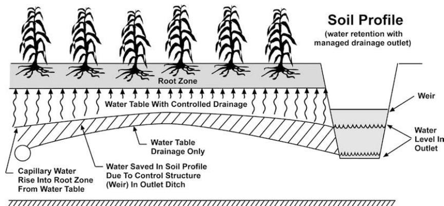
Figure1. Water level fluctuation with a controlled drainage system [1]
