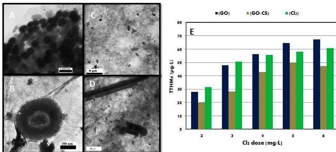
Figure 2: TEM images of GO after coagulation process show the synergistic effect of it on bacteria (A Wrapping, B perturbation of the cell membrane), TEM image of GO/CS binary system wrapping different contaminants during coagulation/flocculation process (C, D), the formation of TTHMs resulting from using different doses of chlorine in case of GO, GO/CS system and Chlorine dosing without coagulant (E).
