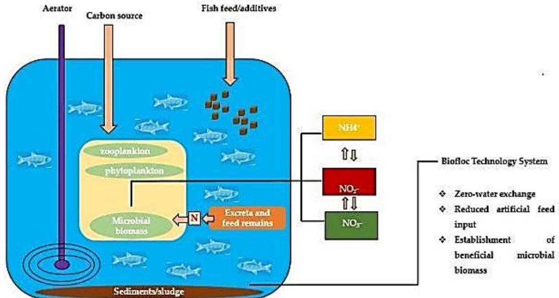
**Figure 1. Schematic diagram of a biofloc technology system**
