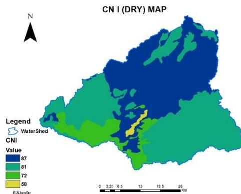
Figure 1. Curve number under the dry moisture condition
