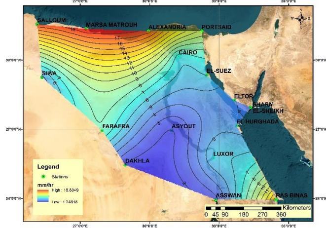
Figure 2. Contour map of rainfall intensity (mm/hr) for storm duration of 0.5 hr and a return period of 10 yr.
