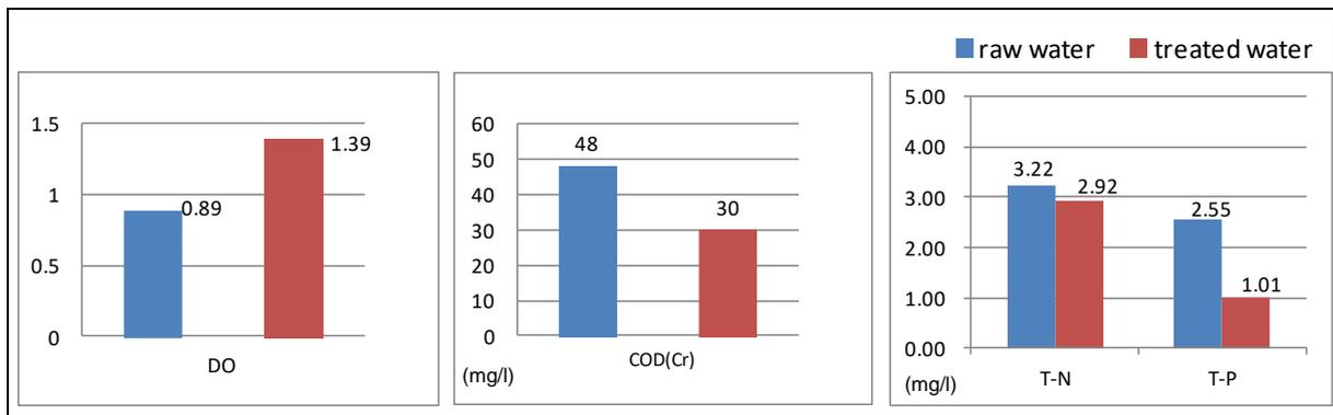
**Figure 2: Comparison of water quality before/after the treatment (In-stream Wetland Treatment facility) in Sandala drain in Kafr Elshiekh Gov.**
