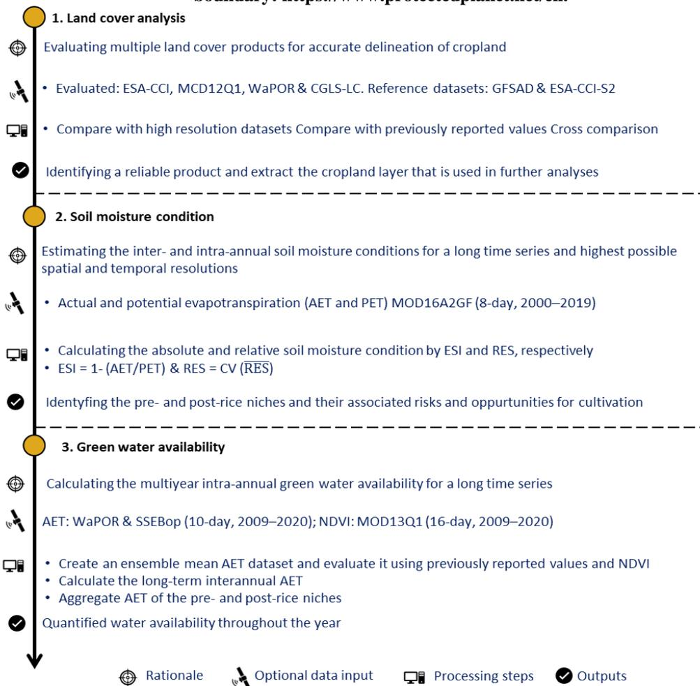
**Figure 2. The developed framework including the main steps, objectives, data used, procedure and output.**
