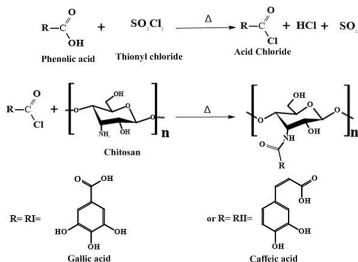
**Scheme 1:** Synthesis of chitosan adsorbents RI and RII
